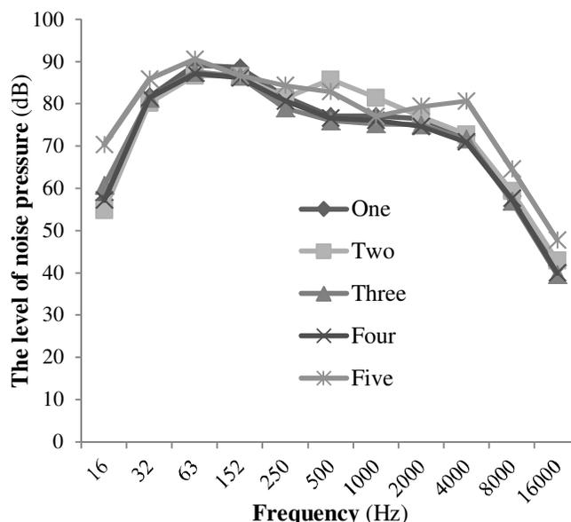
**Diagram 2-** Results of frequency analysis in the position of the driver's ear in different gears in the engine speed of 850 rotations per minute in moving Romanian tractors
