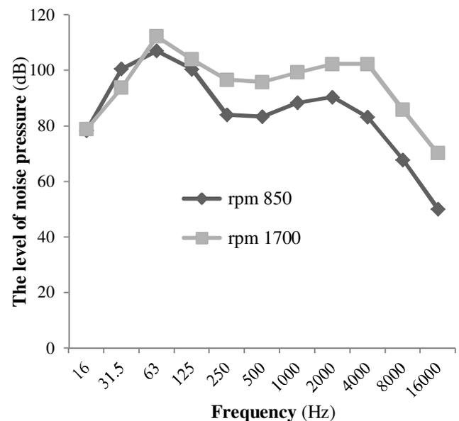
**Diagram 1-** Results of frequency analysis in the position of M-650 Romanian tractor's Exhaust emissions in fixed state in the selected engine speeds
