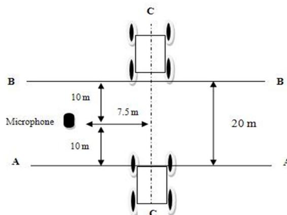
**Figure 1-** Measuring noise level in the position of bystanders of Romanian tractor (M-650)
