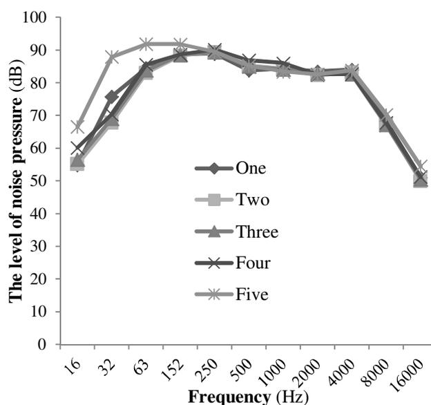
**Diagram 3-** Results from the frequency analysis in the position of the driver's ear in different gears in engine speeds of 1700 rotations per minute in moving Romanian tractor
